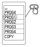
With a beep sound, the contents of the selected program (in this case, PROG1) are copied to the program number displayed on the top of the display (in this case, PROG4).
